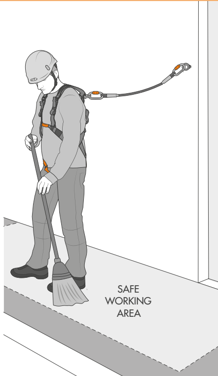
9.2 - Working on a horizontal surface
